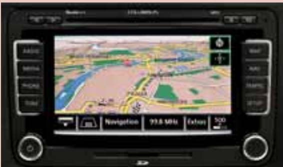
Columbus navigation system: in addition to the functions that are the same as in the Amundsen navigation system*, it offers a 6.5" high-definition colour touch-screen display, a navigation DVD in two versions – for Western and Eastern Europe, a 30GB hard disk (navigation data leave approx. 20 GB of spare capacity which may be used for storing MP3 or WMA music files), fast calculation of a route and its projection due to a high-capacity processor and other functions. In combination with a TV tuner, it also allows watching TV broadcasts or browsing teletext pages.
