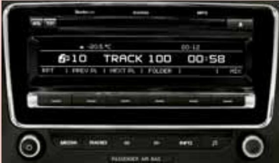
Radio Swing: 2 DIN, AM/FM tuner with RDS and TP systems, dual antenna for FM reception, CD player, connection to a CD changer, CD-MP3 and CD-WMA player, MDI capability, 4x 20W amplifiers, digital signal processor with an equaliser, dot-matrix display conveying data from the Climatronic air conditioning, parking sensors, time and outdoor temperature, compatible with a multifunctional steering wheel, secured by convenient electronic encryption.
