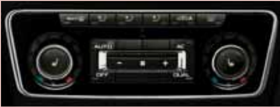
Climatronic – dual-zone air conditioning with electronic regulation, including automatic regulation of the air circulation in the interior. Automatic setup and maintenance of air temperature in the interior as well as intensity and direction of air flow.
