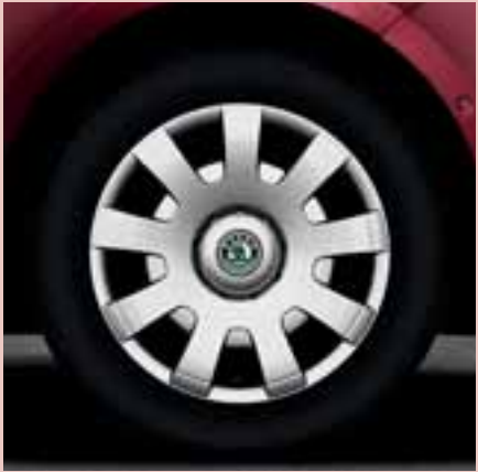
7.0J x 16" steel wheels for 205/55 R16 tyres with Tempel hub covers.
