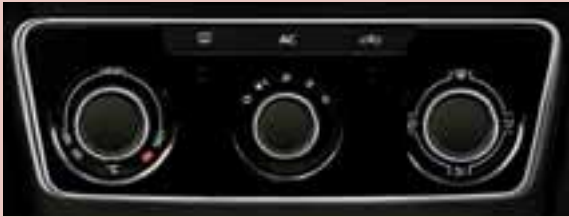
Climatic – air conditioning with automatic regulation: automatic setup and maintenance of interior temperature, manual setup of intensity and direction of air flow.
