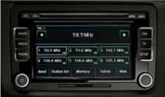
Radio Bolero: in addition to the same functions as the Swing radio, it has, among other things, a memory for radio traffic reports (TIM), an integrated 6-CD changer, 6.5" colour touch-screen display (TFT), a reader for SD or MMC data cards with files in MP3 or WMA formats, compatible with the Sound System; it cannot be connected to a CD changer in the luggage compartment.
