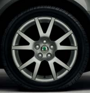
6.5J x 16" Spider alloy wheels for 205/55 R16 tyres (part of the sports package)
