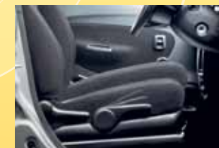
INTEGRATED SEAT HEIGHT ADJUSTER (Available in 1000cc only)
