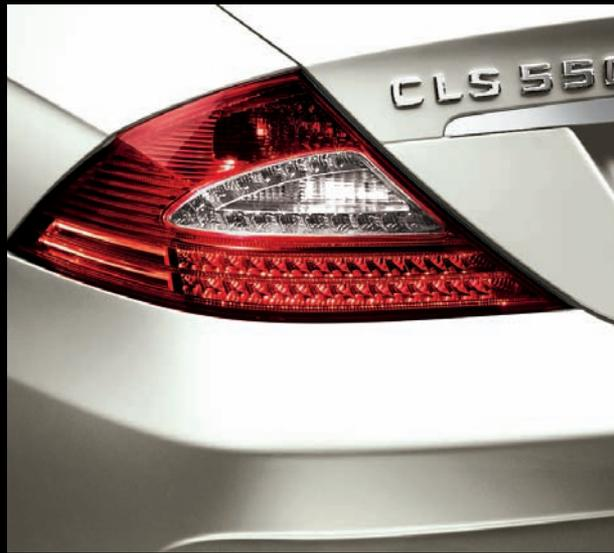
**Responsive.** Brilliant, long-life all-LED taillamps include quicker-illuminating brake lamps. The optional Bi-Xenon headlamps incorporate Active Curve Illumination, whose swiveling beams increase usable illumination of curving roads by up to 90% over conventional fixed headlamps.
