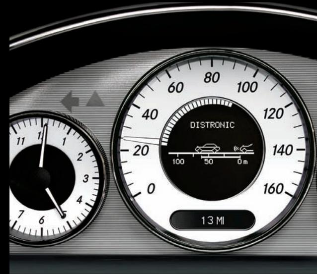
**Attentive.** Optional DISTRONIC adaptive cruise control actively monitors your following distance from the vehicle ahead of you. Originally pioneered by Mercedes-Benz, it can automatically apply the brakes when traffic ahead slows, and resume your preset speed when it clears up.<sup>7</sup>
